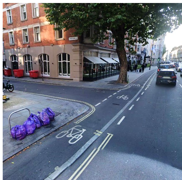
Figure 5: a stepped cycle track with 'flush kerb' entry treatment (Google Maps)
